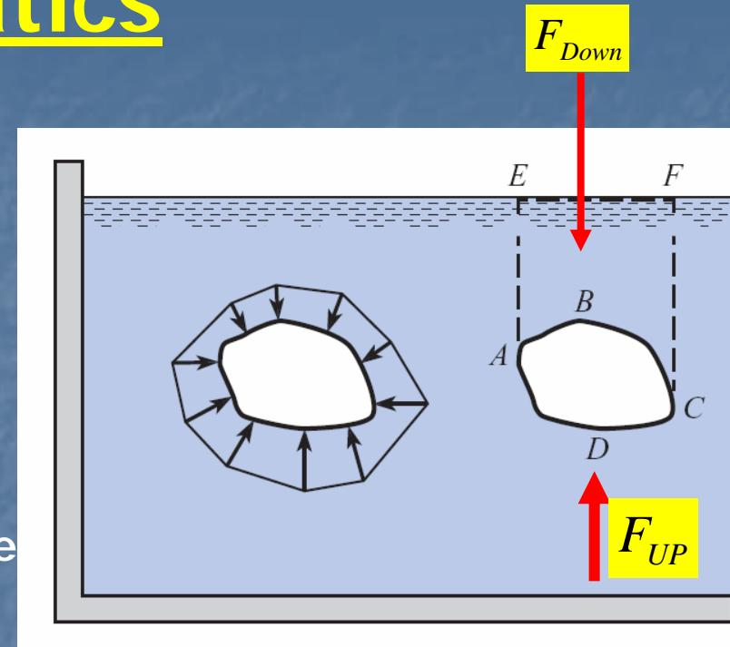
The net force = Buoyant Force =  $F_B \uparrow = \gamma V_{ABCD}$
