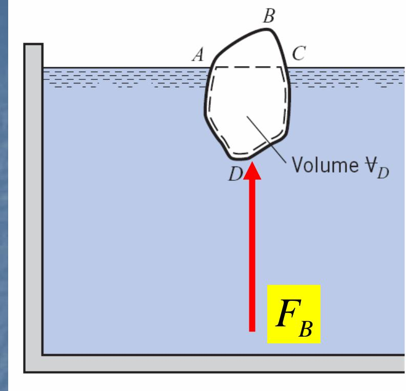
The general principle of Buoyancy is called Archimedes Principle which states that for an object which is partially or totally submerged in a fluid, there is a net up-ward force (buoyant force) equal to the weight of the fluid.
