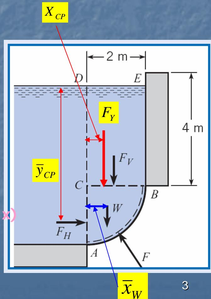
Forces on Curved Surfaces may be found by applying Equilibrium concepts to systems comprised of the fluid in contact with curved surfaces
